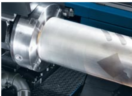
The RotoLas add-on enables you to cut tubes and pipes on your 2D laser cutting system.
