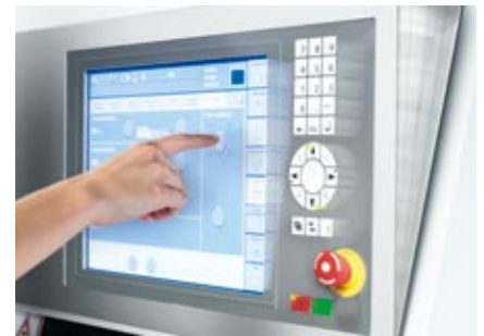
The user-friendly touch screen with intuitive menus can be tilted to avoid reflections.
