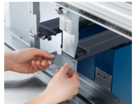
The integrated bending line laser ensures spot-on positioning.
