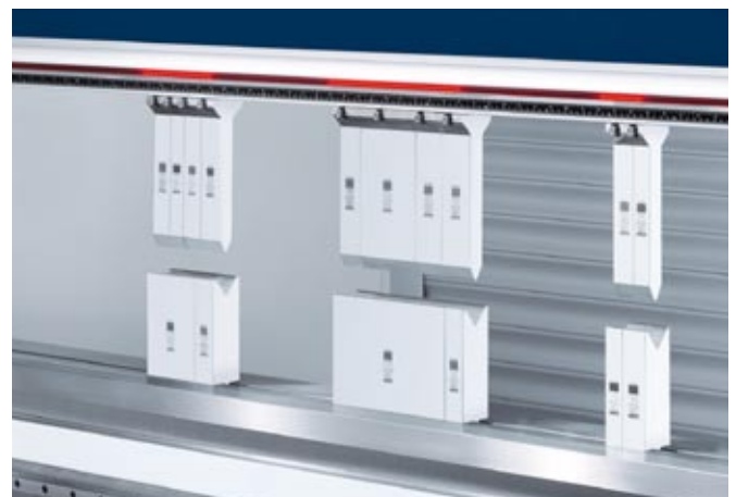
Optical tool setup and positioning aid.
